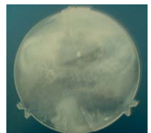
Post annealing & ethanol testing: residual stress: NO, orientation stress: YES
