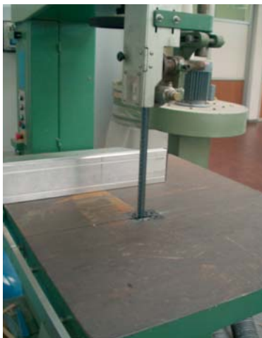
Sprue Cutting by saw
